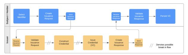
Figure D1: Expanded Credential Issuance Flow with Issuer Steps
