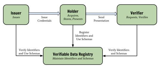
Figure 2: VC Ecosystem diagram from the VC Data Model<sup>9</sup>.
